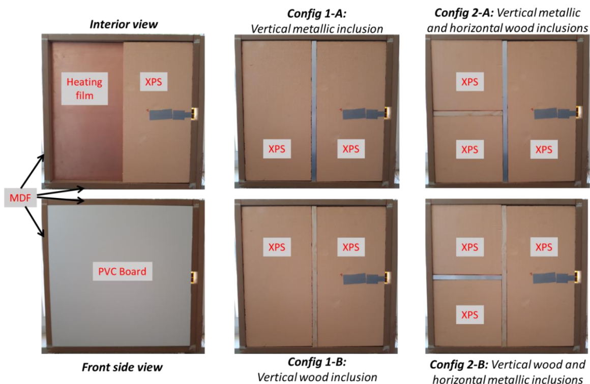
Figure 5.2: Images of the test bench N°2 with different configurations; wood inclusions are pine wood rods; metallic inclusions are aluminum hollow tubes; all inclusions have a square section of 20 mm x 20 mm
